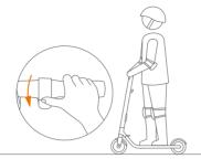
Put your other foot on the footrest to keep both feet stable. Press the throttle on right hand to speed up when you are balanced.
