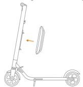
2. Install the support bracket and fasten securely with three screws, as shown.
