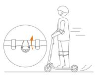
4. Slow down by releasing the throttle;stir the brake handle thumb shifter quickly and stamp the fender with foot at the same time to trigger mechanical braking in order to make a sharp brake.
