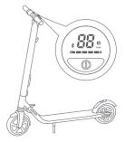
1. Power on the scooter and check the indicator lamp power level. Charge the scooter if the battery level is low.
