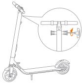
Firmly connect the wires inside the handle and the stem. Slide the handle onto the stem. Be aware of the correct orientation.
